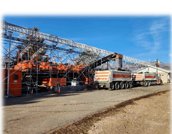
Centrifuges and Conveyors Loading Dewatered Solids into Truck
